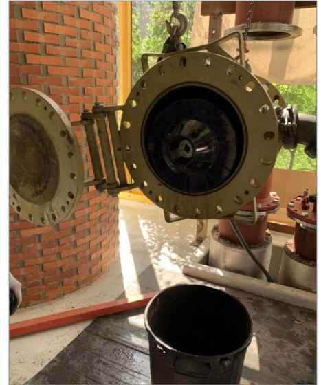
Fig. 19 – Recovery of Quest InVista™ Inspection Tool from Pipework
