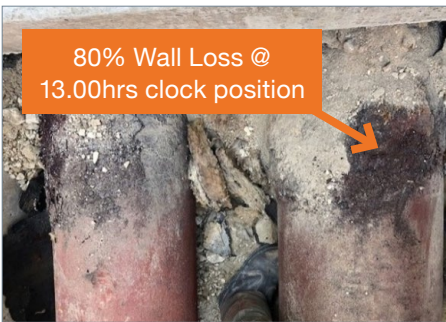
Fig. 23 – Visual confirmation of defect following excavation.
